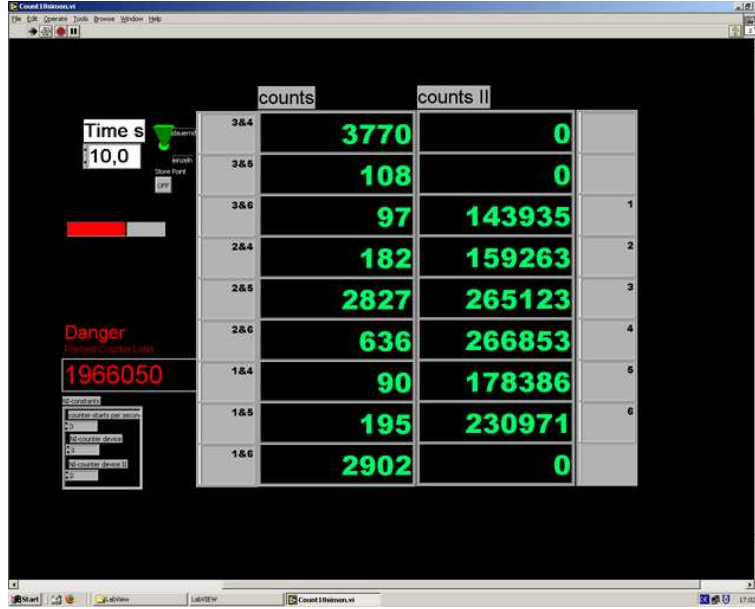
Figure 6.3.: Typical count rates per 10 s for the experimental violation of the Bell inequality and the experimental qutrit quantum key distribution. The left column shows the coincidences, where the three perfect correlated count rates are easily distinguished from the rest. In the right column are the single counts of the six detectors.
