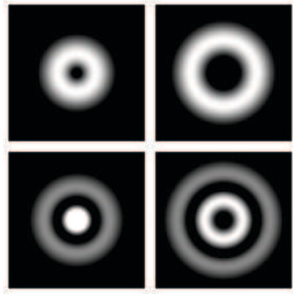
Figure 4.4.: Numerically calculated Laguerre-Gaussian modes with different indices p and l . The upper left is an LG_{0,1} mode and the upper right an LG_{0,3} mode. Due to their characteristic intensity profile, these modes are called doughnut modes. LG_{0,3} is a mode with a slightly bigger phase singularity compared to LG_{0,1} . In the lower pictures two radial nodes can be observed because of a non-vanishing index p = 1 , where the left is an LG_{1,0} and the right an LG_{1,2} mode.
